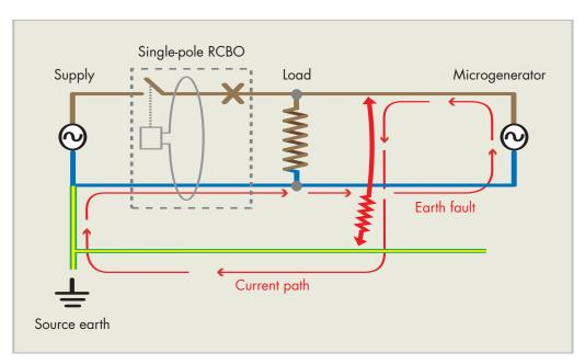
It should be noted that, if the RCD element of the RCBO has been provided for additional protection against electric shock, this arrangement is not permitted and the RCBO would need to switch both line and neutral conductors (see (ii) above).
