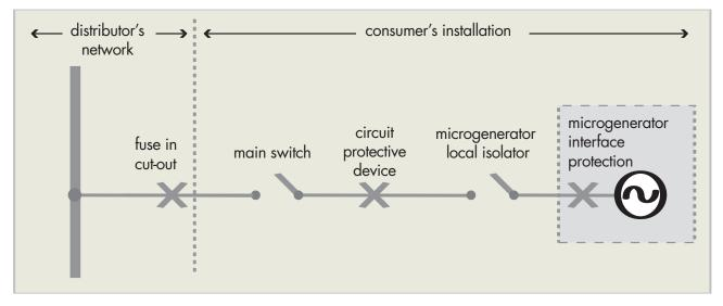
Example of circuit diagram for a microgenerator installation
